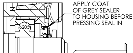
PULLEY END DETAIL
